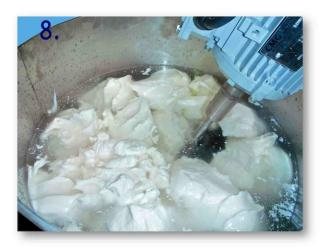
After 2-3 minutes of a 5 second ON/OFF sequences, the product should be thick enough to leave the motor on for about 5-6 minutes; however an eye should be kept on the mixing process so that the motor can be stopped if a vortex forms.
